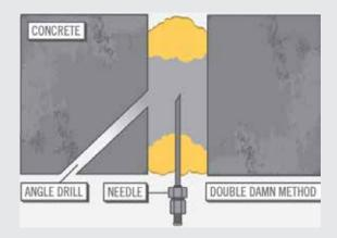
If leak flows are high, one or more pieces of small diameter pipe can be embedded in the packing material. These nipples serve to relieve pressure and divert flow while the packing seal solidifies. Once the seal has cured, a small amount of resin injected through the nipples will rapidly complete the seal. The pipe nipples can then be removed.
