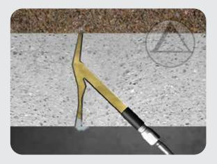
Hold pressure constant for several minutes. If flow still does not occur, raise the pressure slowly. An extra minute or two can make the difference between 95% and 100% crack filling. Sudden applications of high pressure may help unintentionally open the crack. If in doubt, **slower is better**. As soon as flow is established, decrease pressure as much as possible consistent with desired flow rate.
